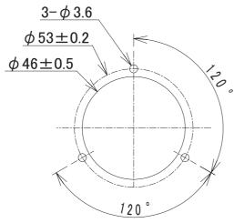
Thickness of the Panel :  $\leq$  3 mm Recommended Torque for fastening the nut : 0.4 ~ 0.5 N·m (4~5 Kgf·cm)
